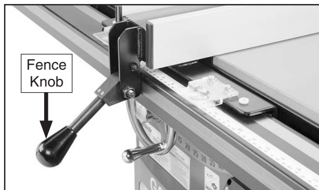
Figure 42. Fence knob installed.
